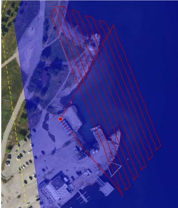
Figure 7. Flight pattern example DJI Matrice 600. Photo: Medyan Ghareeb, Drone Logbook.
