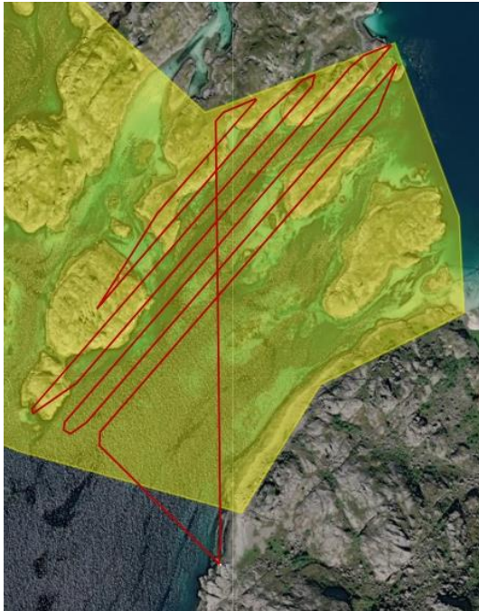
Figure 5. DJI Matrice 300 Flight Pattern Example. Photo: Medyan Ghareeb, Drone Logbook.
