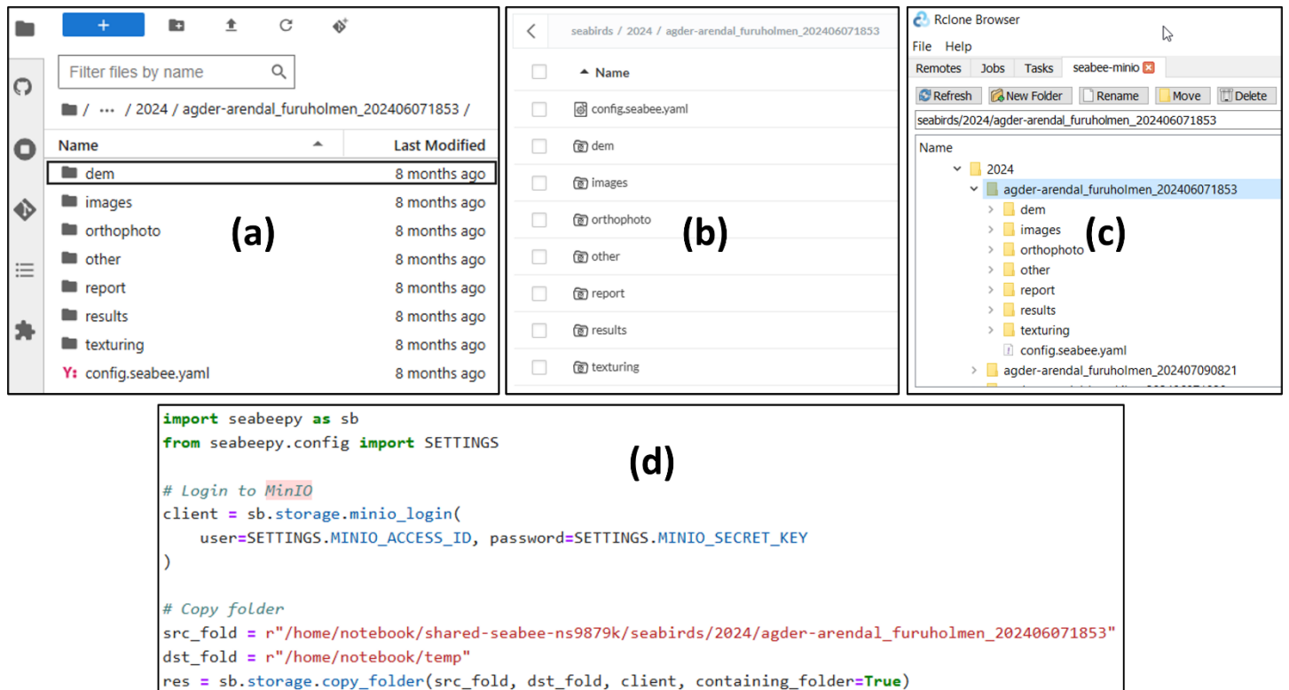
Figure 3: Four different options to access the same SeaBee data. (a) JupyterHub file browser; (b) MinIO web interface; (c) RcloneBrowser from an external machine; (d) Programmatically via Python using seabee.py .
